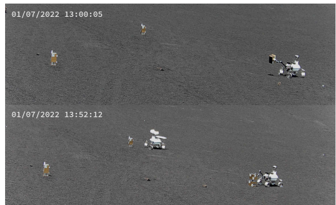
Figure 9: Images from the lander camera during the autonomous deployment of the power payload box (top) as well as the LOFAR payload box (bottom) with the LRU2 rover.
