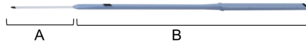
Figure 2: Cryotop ® cryodevice comprises an (A) embryo carrier where an embryo is placed, attached to a (B) plastic handle.
