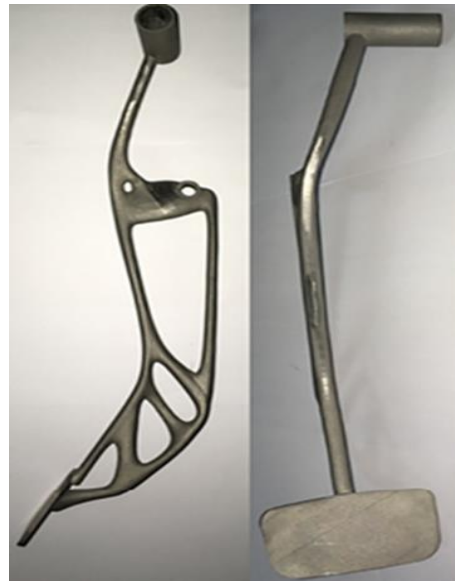
Figure 17. Metal brake pedal using BASF Ultra fuse 316L metal-polymer filament via FDM. Adapted with permission from Sargini et al. [9]. 2021, Elsevier.
