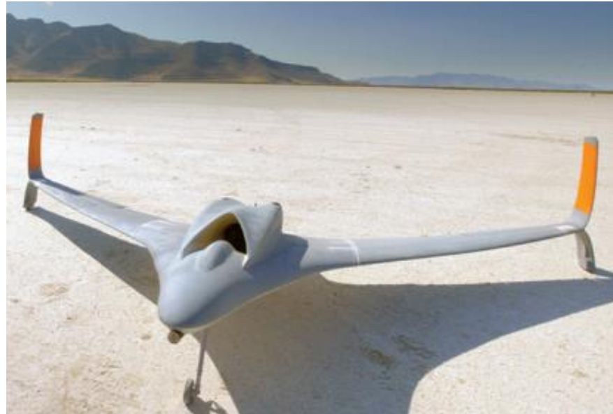
Figure 16. UAV using the FDM process. Adapted with permission from Stratasy's [202].
