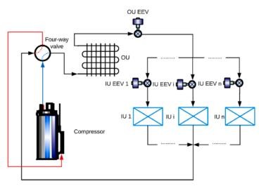
Figure 2. Simplified VRF diagram [5].
