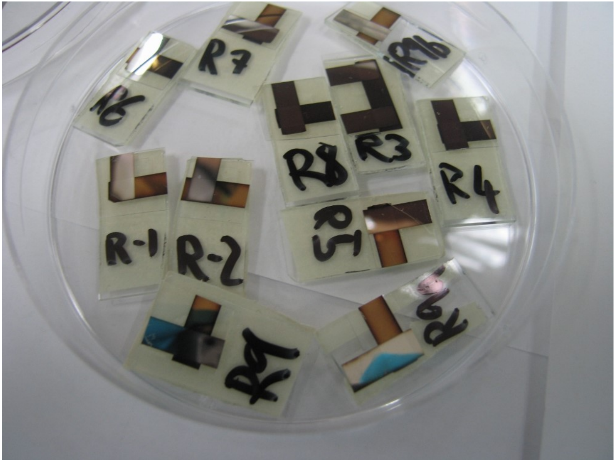
Figure 2: Memristor devices used in this work, shown in a petri dish for scale. These devices were sputtered onto plastic, but mounted on glass slides for testing
