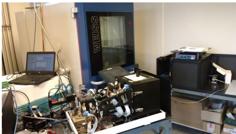
Figure 6.22 Setup of the temperature chamber test, where the RF generator was the only device inside the temperature chamber.
