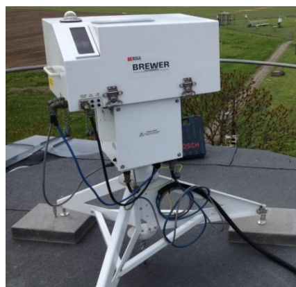
Figure 1.24 Brewer spectrophotometer model MKIII (double monochromator) mounted on a solar tracker.
