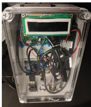
Figure 4.13 Waterproof case contains the TE controller of the AOTF, environmental sensors, and an Arduino as a modulation signal generator.
