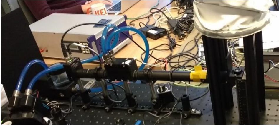
Figure 6.1 Solid-state spectrometer performing measurements of a 50W halogen lamp at Kipp and Zonen Facilities.
