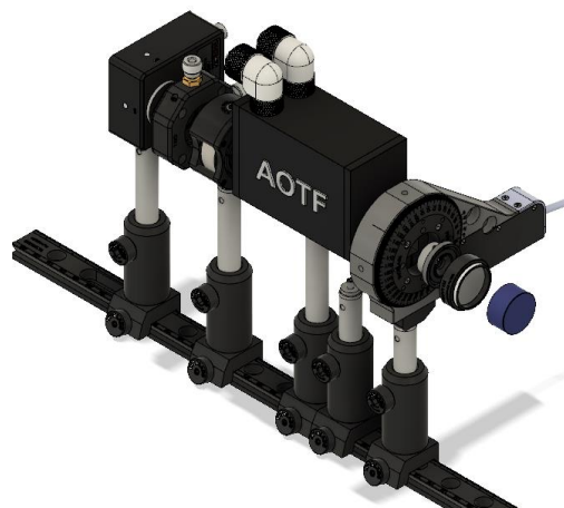
Figure 4.3 The image displays a 3D model of the AOTF spectrometer.
