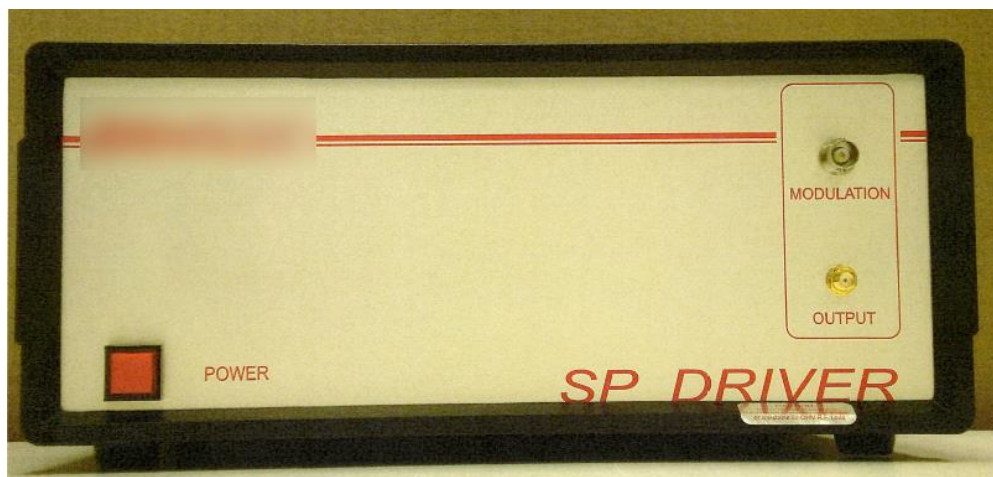
Figure 4.14 Picture of the RF controller used in this project (300 mm wide, 150 mm high, 280 mm deep).
