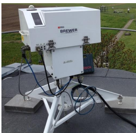
Figure 1.17 Brewer spectrophotometer model MKIII (double monochromator).
