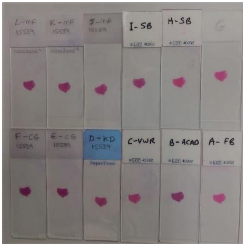
Figure 3. 5 A series of prostate tissue sections from the same BPH patient are mounted on 12 different types of glass slides.
