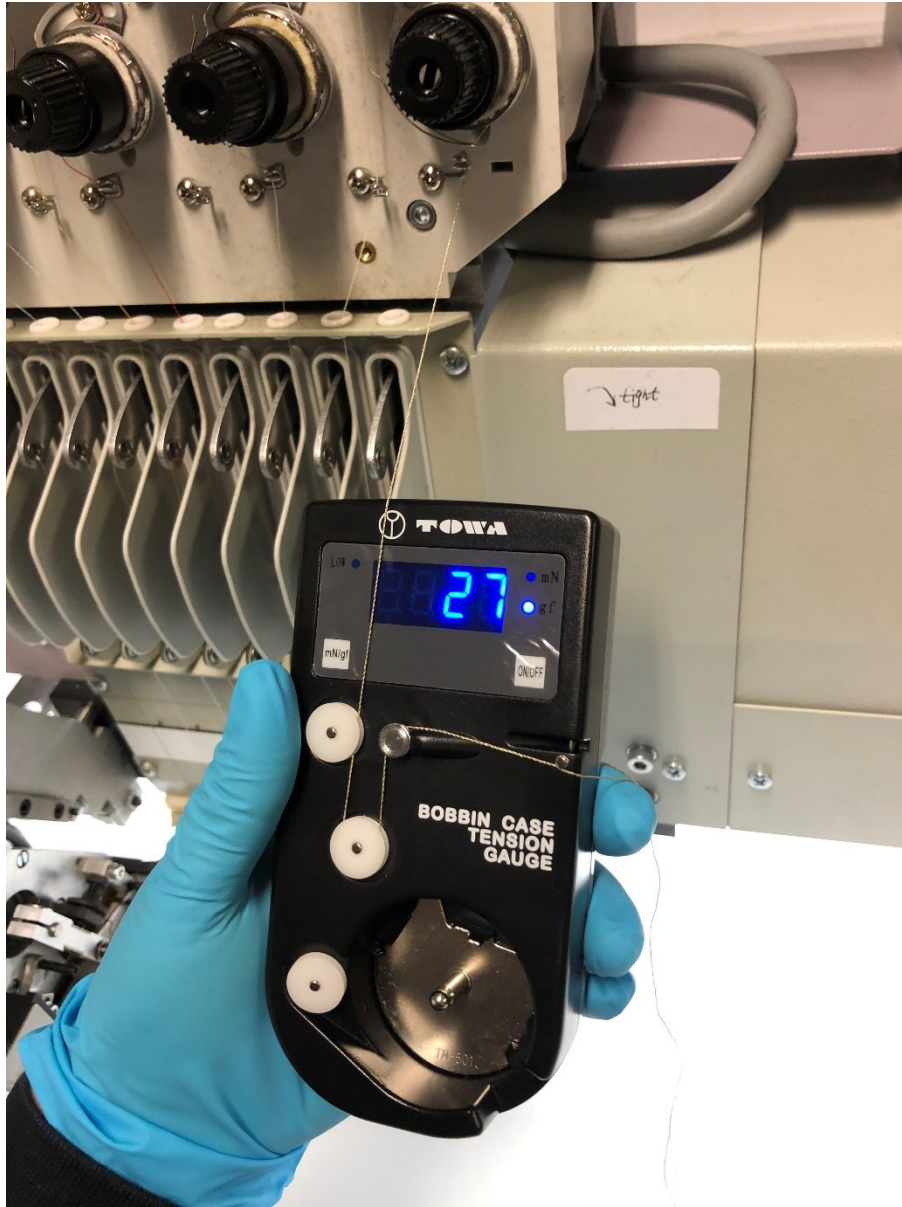
Figure S3-3. Needle thread pre-tension measurement with digital tension gauge.
