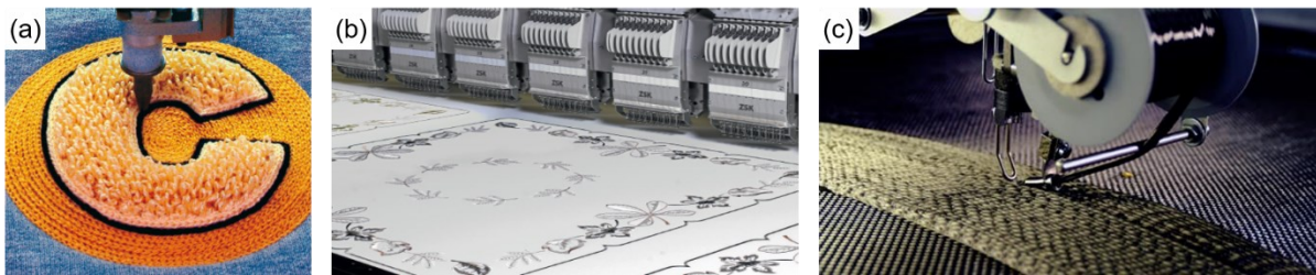
Figure 2-2. ZSK embroidery machines. (a) Chain-stitch embroidery/ K-Head series; (b) Multi-head standard embroidery/ F-Head series; (c) Tailored fibre placement/ W-Head series [63].
