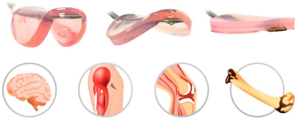
Figure 8 Fmoc-based peptide hydrogels with tuneable stiffness to mimic different human tissues for TE applications. Soft hydrogels (0.8-1.1 kPa, left) can be used to mimic very soft tissues such as brain; medium soft (3-4 kPa, middle) and stiff hydrogels (8-9.2 kPa, right) can be used for harder musculoskeletal tissues such as muscle, cartilage or bone. Adapted from Biogelx.
