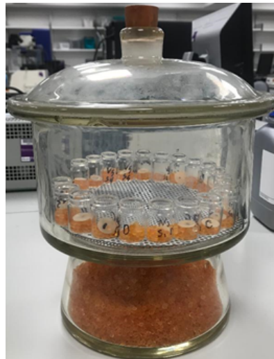
Figure 3-10: Desiccator used in this study to store specimens during desiccation and reconditioning cycles.
