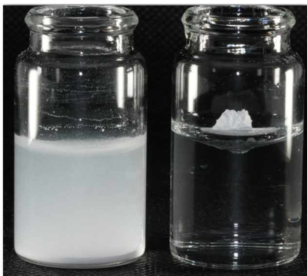
Figure 3-16: Barium borosilicate glass sinks in water (left), the salinized Barium borosilicate glass floats (right).
