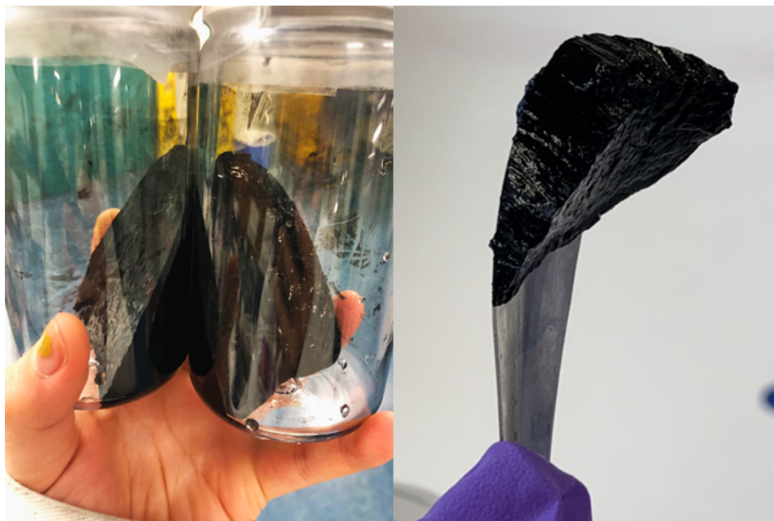
Figure S2 Image of 3D printable inks showing the viscous nature. Inks have been printed through nozzles as small as 250 \mu\text{m} in diameter, and extruded filaments were strong enough to support their own weight and 25 subsequent layers without deflection (printed wet structures in Fig. 2g ).
