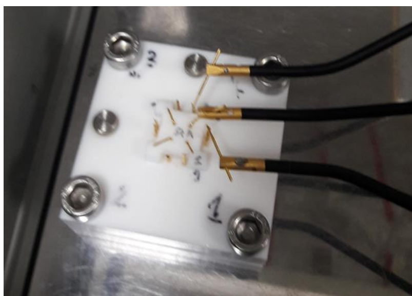
Figure 121 Assembled measurement system inside a probe station and the contacts are connected to the electrical measurement system.
