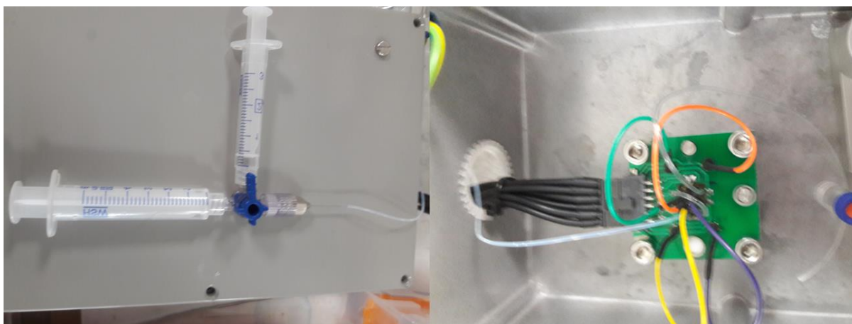
Figure 120 The set up used for flow cell measurements. A three-way stopcock tap is connected to two syringes containing the prepared fluids needed for the experiment. The syringes are mounted on to separate syringe pumps allowing the flow rate to be controlled. Only one syringe pump is used at a time. The fluid is introduced into the cell through by PTFE tubing connected to the stainless-steel inlet tube. The system dead volume (including the three-way stopcock and tubing) was \sim 150 \mu\text{l} .
