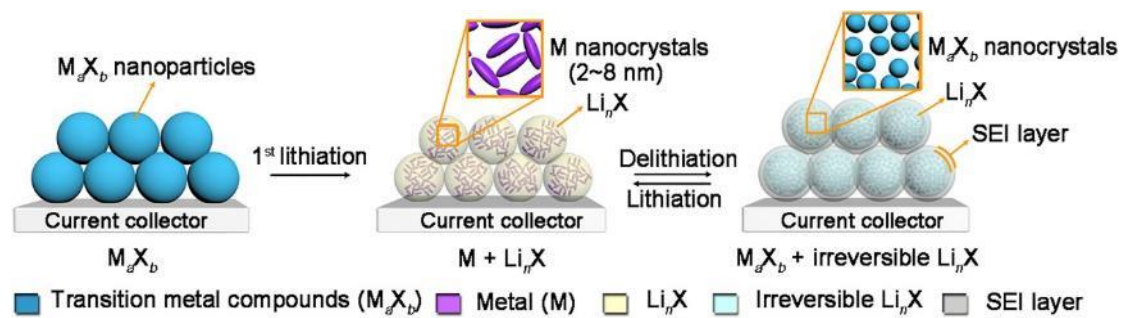
Figure 1.13. Schematic of the local chemistry transformation of transition-metal compounds during the conversion reaction. Reproduced from [101].
