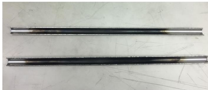
Figure 5-12 Carbonised inner surface of heating pipe after a 750 °C thermal fault with MIDEL 7131
