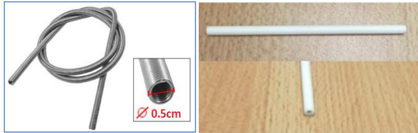
Figure 4-2 Heating element components: (a) Kanthal A-1 coil; (b) ceramic insulator.
