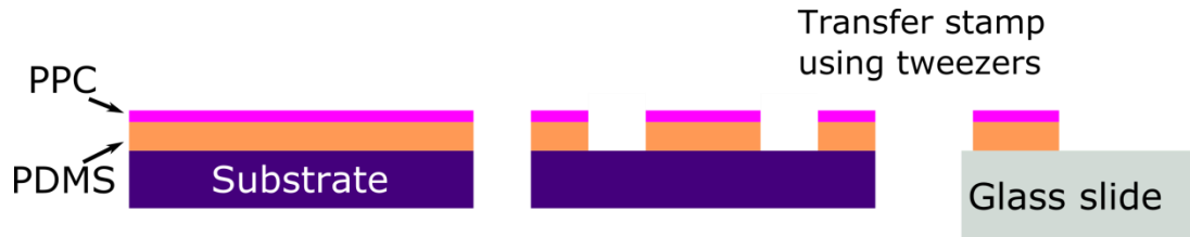
Figure 15: Preparation of a PDMS/PPC stamp. A piece of commercial PDMS is placed onto a substrate and cleaned using oxygen plasma. PPC is spin-coated on top and baked. The PDMS is cut into 2-5 mm squares and moved onto a clean glass slide using tweezers.
