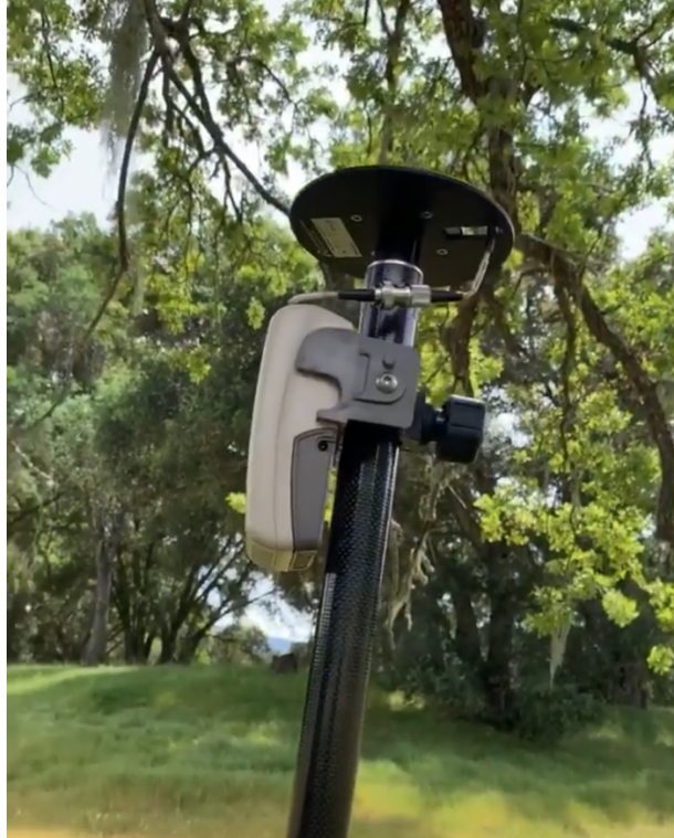
Figure 18. Arrow Gold GPS device assembled in the field.
