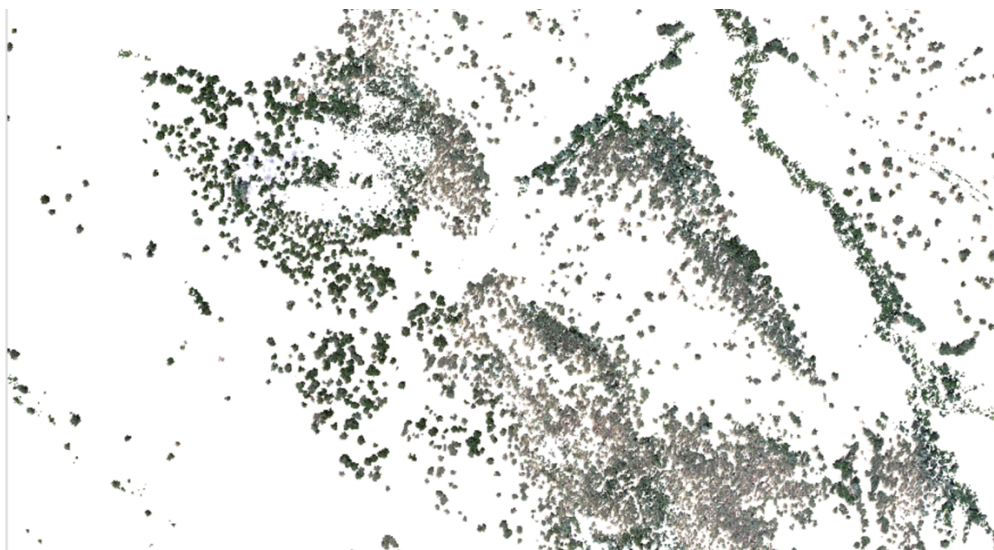
Figure 22. The NAIP imagery clipped to the locations of the trees found using the canopy height model from LiDAR data.
