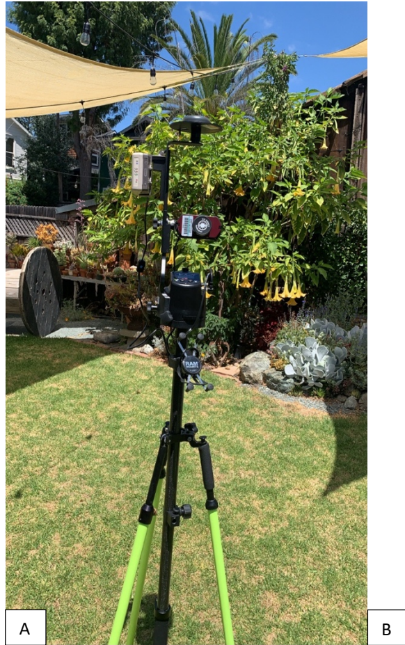
Figure 19. A. The fully assembled laser and angle device using all of Dr. Andrew Fricker's equipment. B. Photo of assembled device from the Laser Offset Mapping with Collector Manual. Some set-up steps are slightly different based on the parts Dr. Fricker has but the overall idea is the same.
