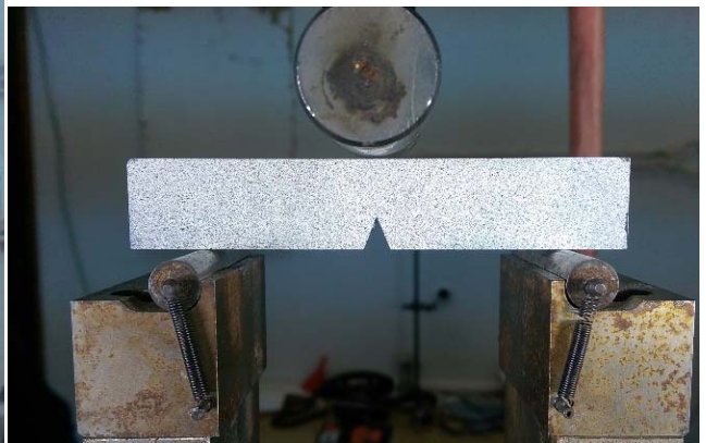
Figure 3. The prepared specimen, prior to loading
