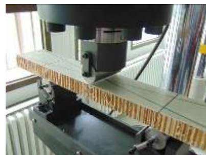
Figure 15. Three point bend test setup
