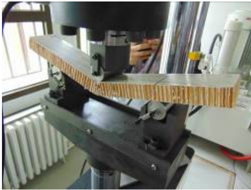
Figure 17. Loaded beam before top plate failure
