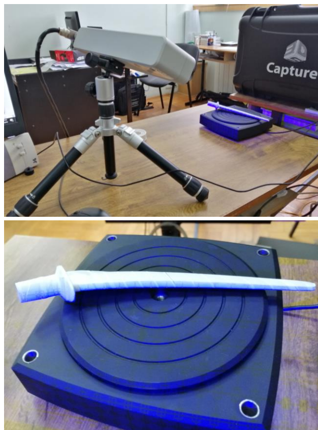
Figure 2. 3D scanning procedure of total hip replacement implant (above - device, below - physical model on scanning platform).
