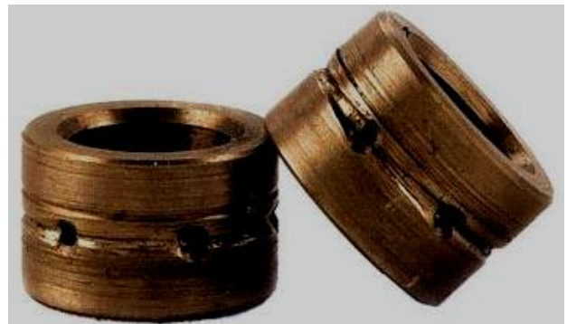
Figure 8. Radial bearings damaged by dirty oil
