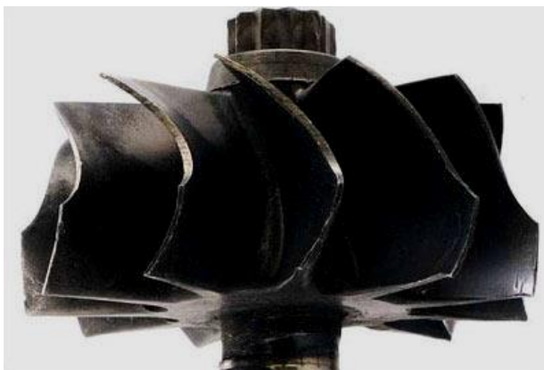
Figure 4. Rotor damaged by foreign objects with soot build-up
