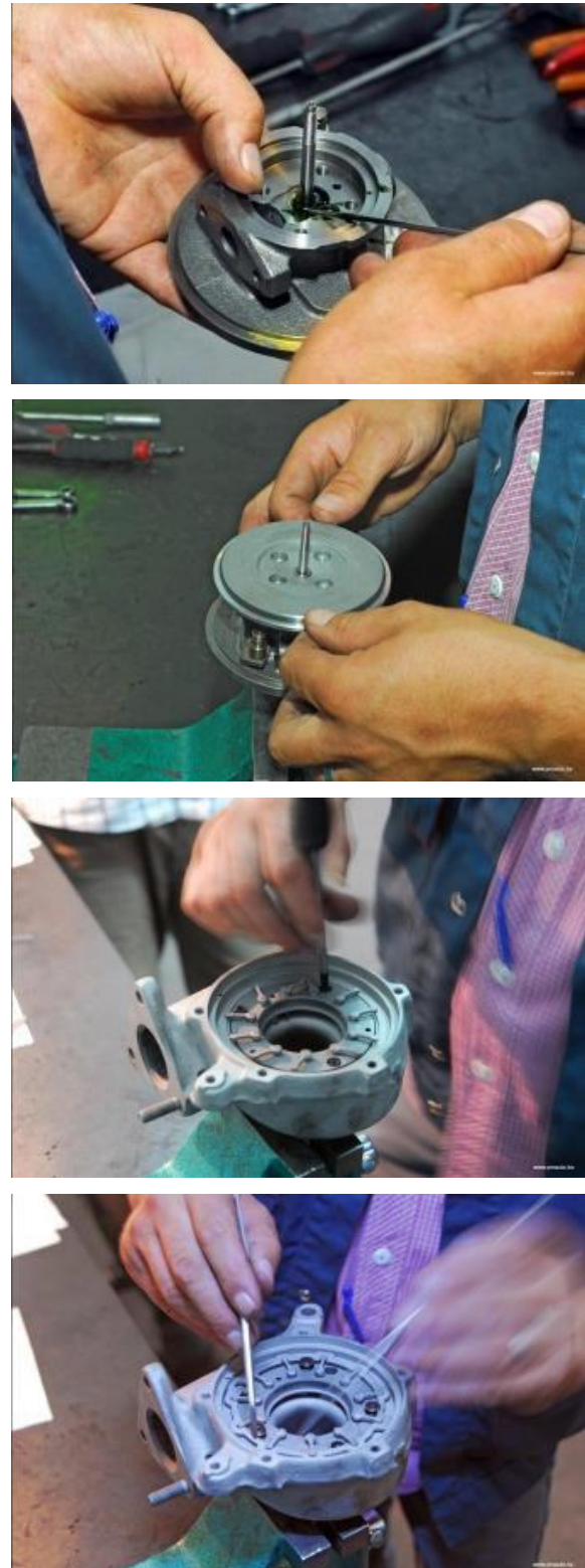
Figure 17. Reconditioning of turbine parts [1]
