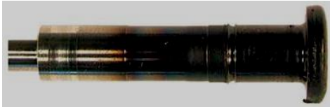
Figure 10. Damage to the turbocharger shaft due to lack of lubrication
