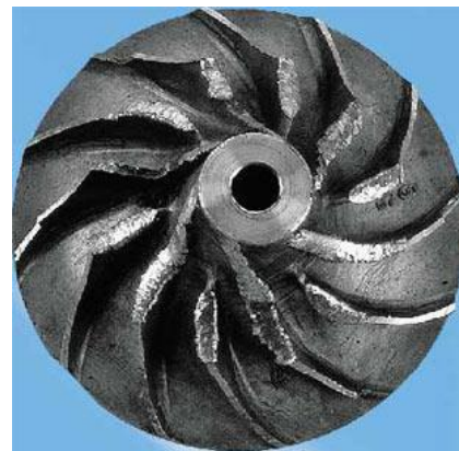
Figure 1. Compressor wheel damaged by a foreign object
