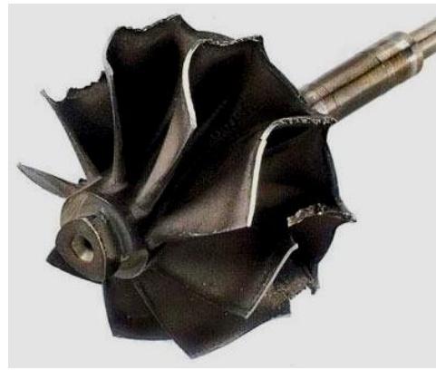
Figure 5. Rotor damaged by foreign objects
