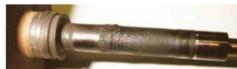
Figure 12. Effect of high temperature on the turbocharger rotor
