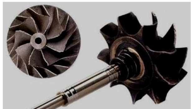
Figure 6. Damage to the turbocharger rotor due to blockage in the exhaust pipe
