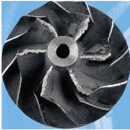
Figure 2. Compressor wheel damaged by a large foreign object
