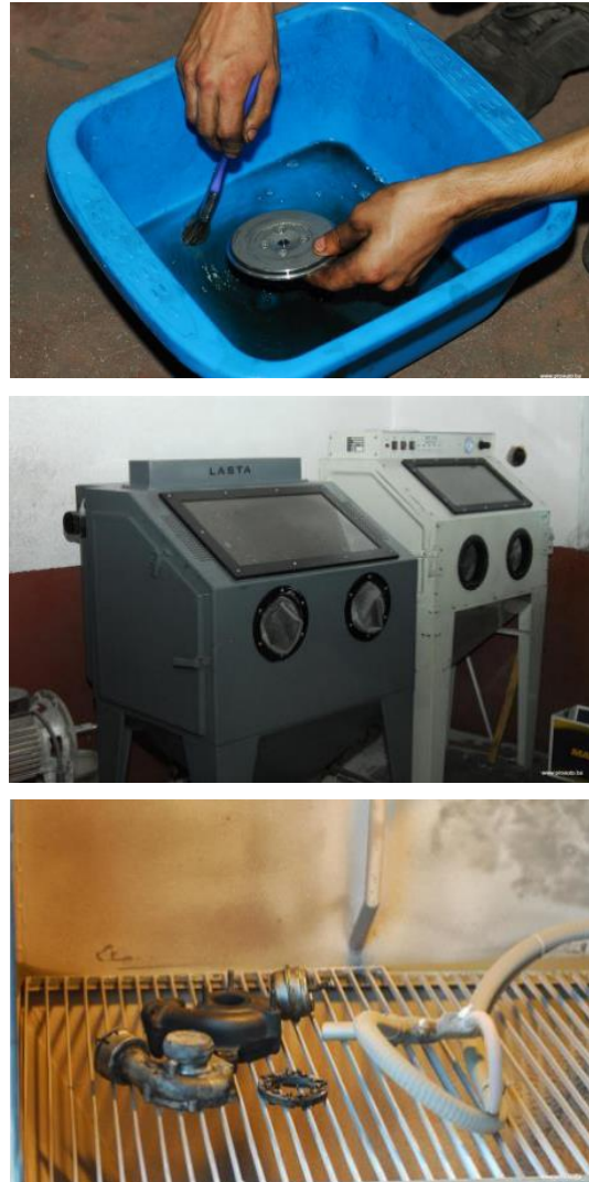
Figure 15. Cleaning, degreasing and sandblasting [1]
