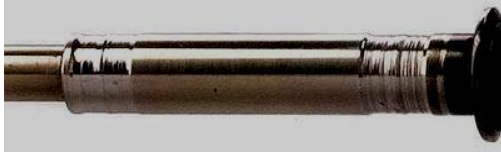
Figure 9. Damage to the turbocharger shaft caused by dirty oil
