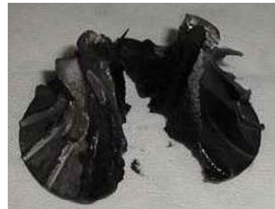
Figure 11. Typical fracture of the turbocharger impeller
