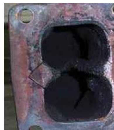
Figure 13. Cracks in the turbine housing due to a high exhaust gas temperature
