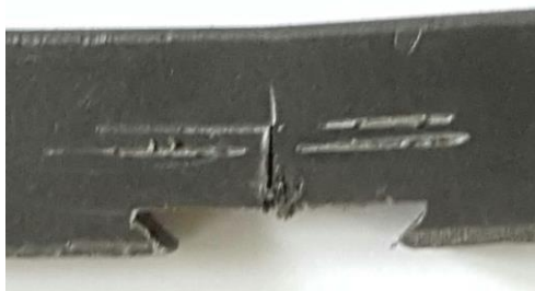
Figure 5. Specimen with crack.
