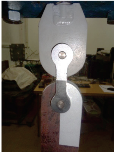
Figure 13 Connecting lug positioned for measurement
