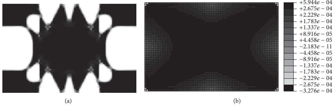
FIGURE 3: Topology optimization result and the modal principal strain of a simply supported plate: (a) topology optimization result from [14]; (b) modal principal strain.
