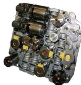
Figure 12: Electro-hydraulic control unit for DCT [11]
