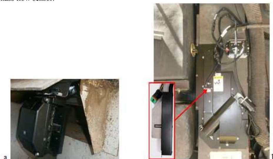
Figure 1. a. Gap between elevator and auger for clear grain and impact plate of mass flow sensor with modul (view from grain tank), b. grain moisture sensor
