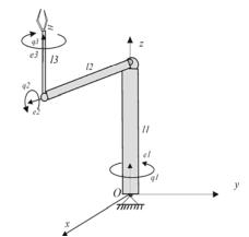
Figure 5. The robotic system with 3 DOF in the reference configuration
