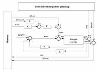
Figure 4. Block diagram of the feedforward-feedback  $PD^{\alpha}$  type of ILC for a robotic system
