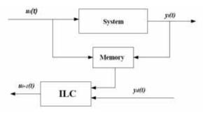
Figure 1. The basic scheme of iterative learning control
