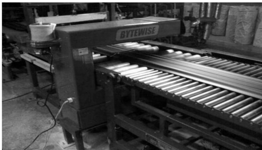
Figure 4. Machine for 'In Line' measurement of profile shape and dimensions.
