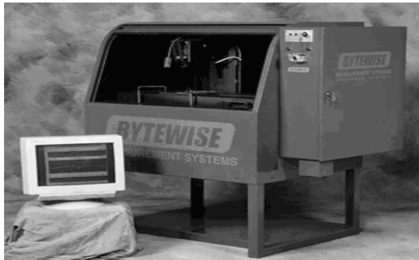
Figure 1. Bytewise machine for 'off line' measurement of profile shape and dimensions
