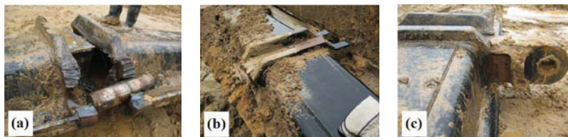
Fig. 2. Fractured (a) female lugs; (b) male lug; (c) chain link body
