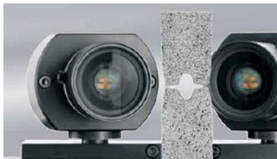
Figure 13 Continuous stereometric recording in laboratory conditions, testing of the tensile specimen type M(T) [5]
