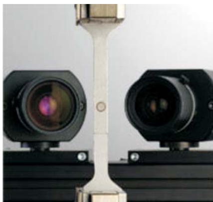
Figure 4 Video cameras "Aramis" with the tested sample at the centre [5]
