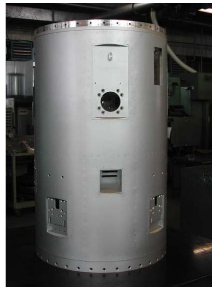
Figure 6. Structure of the GNC Module (prototype)
