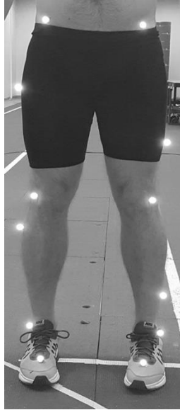
553 Figure 3: Subject positioned for standing calibration trial with retro-reflective marker 554 placed at relevant sites (heel and PSIS are posteriorly positioned). This is to establish local 555 coordinate system relative to global that is marked via static and dynamic calibration with 556 the wand.
