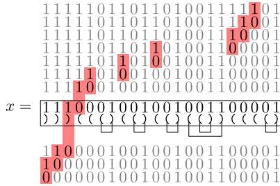
Fig. 4. Construction of the Greene-Kleitman SCD containing a bitstring x via parenthesis matching. The highlighted bits are the leftmost unmatched 0 and the rightmost unmatched 1 in each bitstring.
