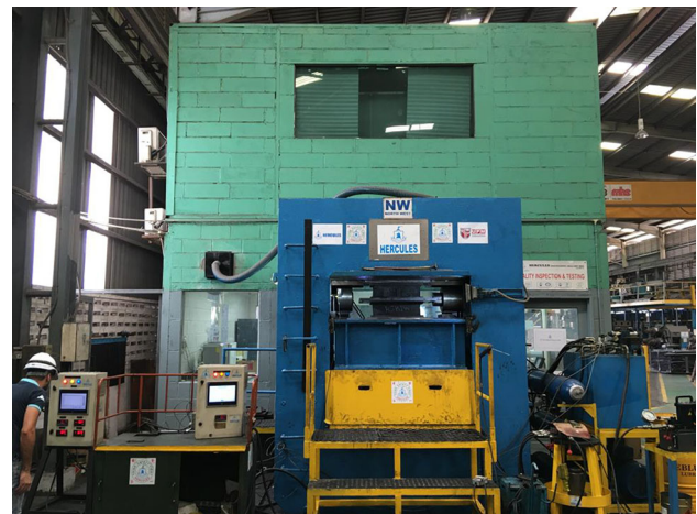
Fig. 9 Overall view of the testing machine and PLC system
