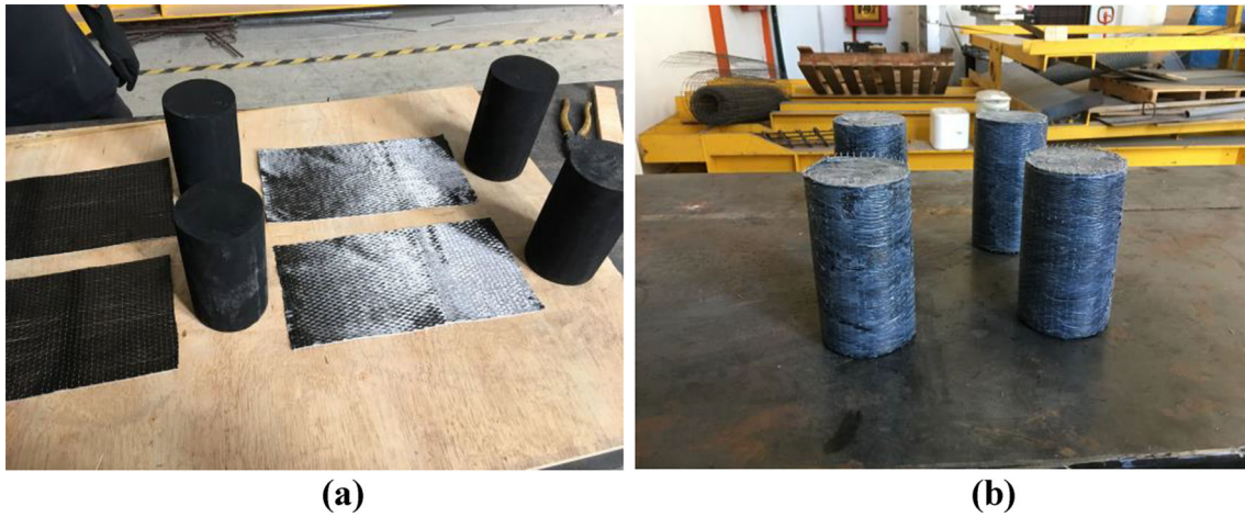
Fig. 6 Four cylindrical rubber cores a before and b after confinement with CFRP sheets
