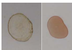
Figure 3-28 Deposition of Zn-PpIX (left) and ZnTPP (right) THF solution on the PVDF substrate, the Zn-PpIX are crystalized on the film, form unevenly died area.
