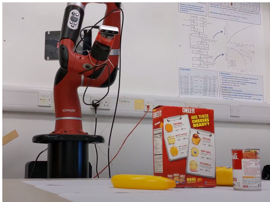
Figure 2.5: A robotic arm that can be used to interact with household objects in an environment. This setup is typical for object-centric tabletop scenes in visual recognition tasks such as object localization, detection, or segmentation. The objects of interest are the camera's main focal point which is attached to the robotic arm.
