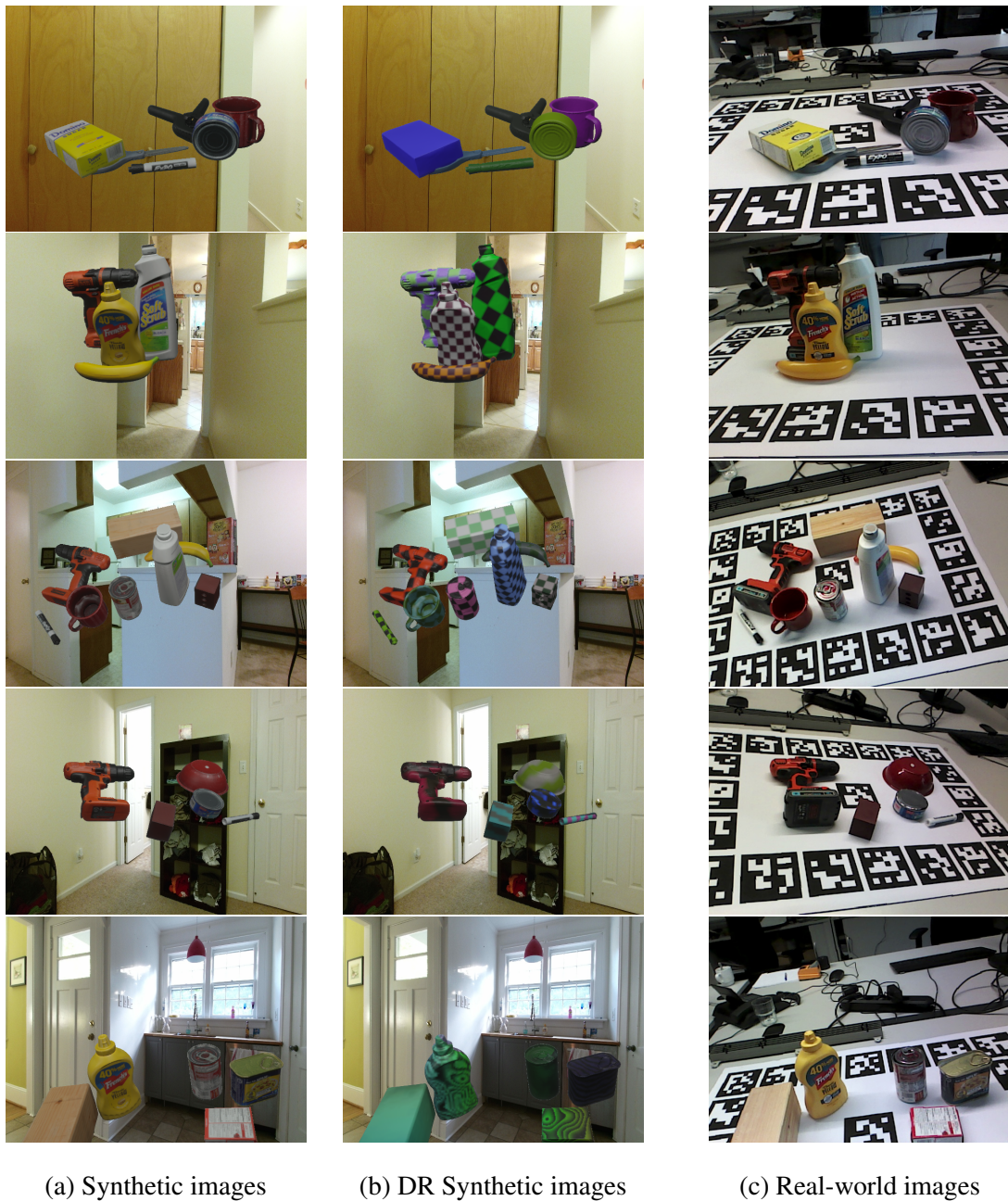
Figure 6.2: We show sample images from the SRDR dataset displaying synthetic (left column), DR synthetic (middle column), and real-world images (right column). The DR images use all the most commonly applied texture randomization techniques in the existing literature and were using real-world backgrounds from the Active Vision dataset [4].
