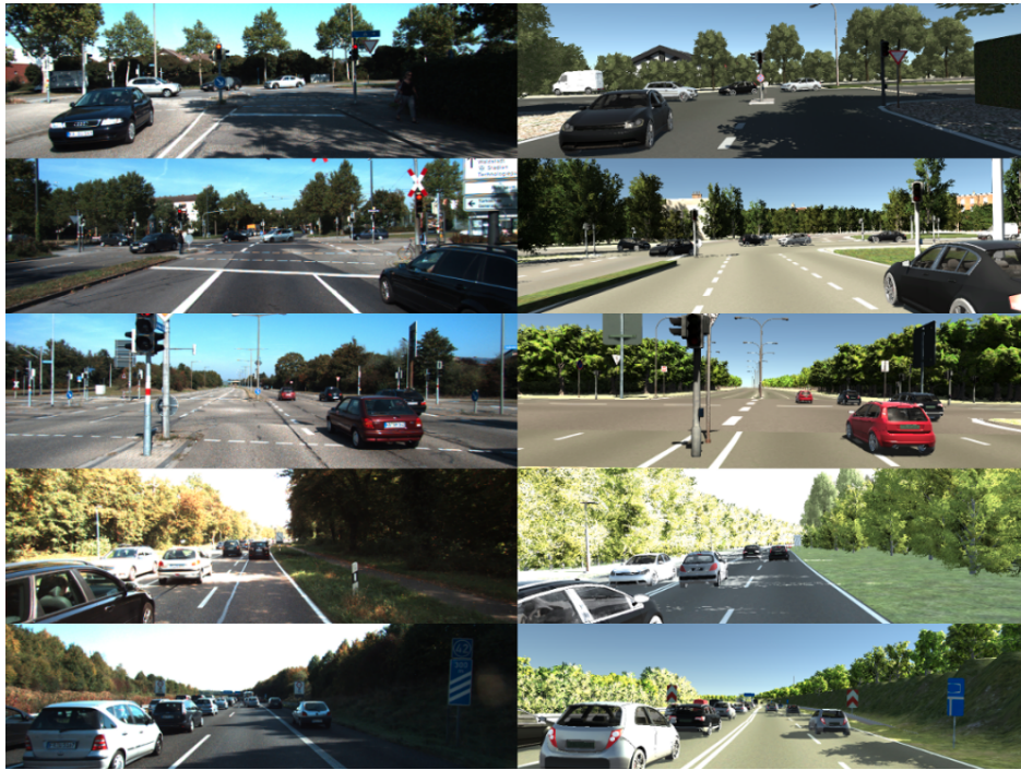
Figure 3.6: Images were taken from Gaidon et al. [54]. The figures show five real-world scenes on the right from the KITTI dataset [57], and five matched synthetic scenes from the VKITTI dataset [54] on the left. The matched artificial scenes differ visually from the real-world scenes, such as the lighting (global illumination appears to light up the entire scene compared to the real-world images), textures and material properties used on the cars, or softer shadows in reality.
