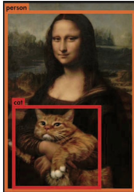
Figure 2.8: Example of an object detection task, where a model was tasked to detect certain classes from a given image. Image taken from Redmon et al. [165]. The bounding boxes define the positions of the objects of interest, while the labels “person” and “cat” describe what appears within the region.
