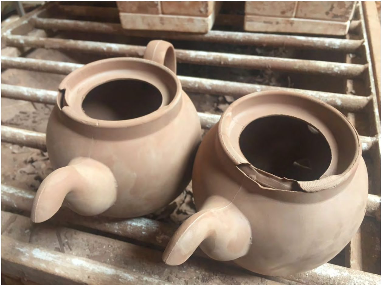
Fig. 128. Airbubbles trapped in the mould on the casting bench in CC.
