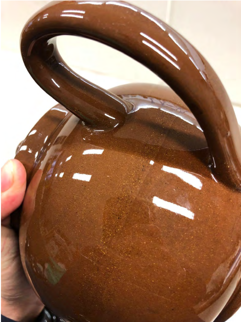
Fig. 81. ALB BBs, visible seam lines on the body of the teapot reveal the split mould manufacture; Ian McIntyre collection photographed in studio.
