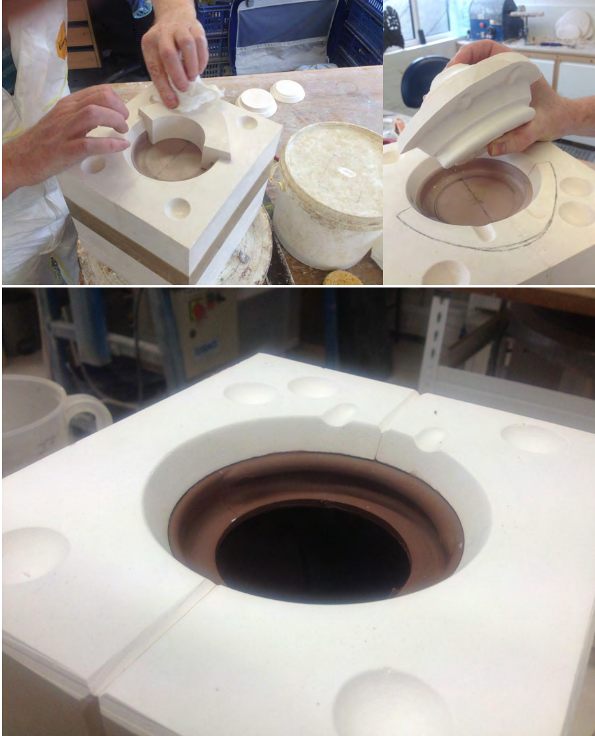
Fig. 120. The loose lump moulding detail that myself and Ed Bentley developed in his workshop. The small part slides out along the two ridges preserving the clay ridge before the main body of the mould is split in two.
