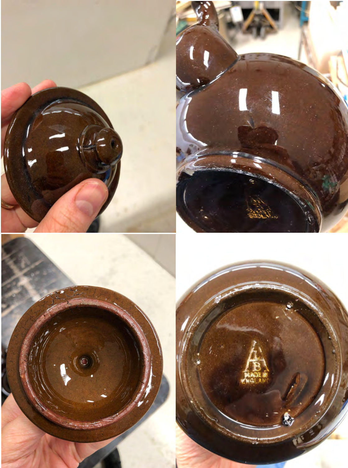
Fig. 83. ALB BBs above, imperfections remain in the teapot, such as a seam line on the finial of the lid and cracking on the internal surface (top and bottom left) and dents, flecks and inclusions of clay in the body of the pot (top and bottom right); Ian McIntyre collection photographed in studio.
