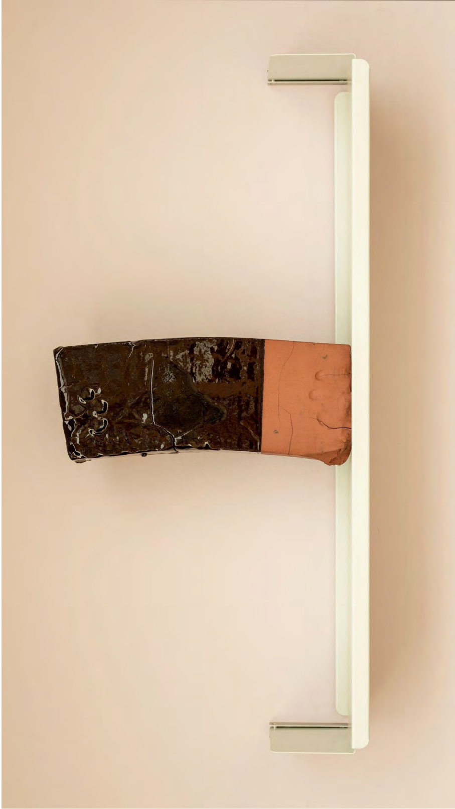
Fig. 74. Object illustrating the red clay and Rockingham glaze: Extrusion, taken from the production line at Valentines Clays and dipped in Rockingham glaze. Image by Geof Howe.
