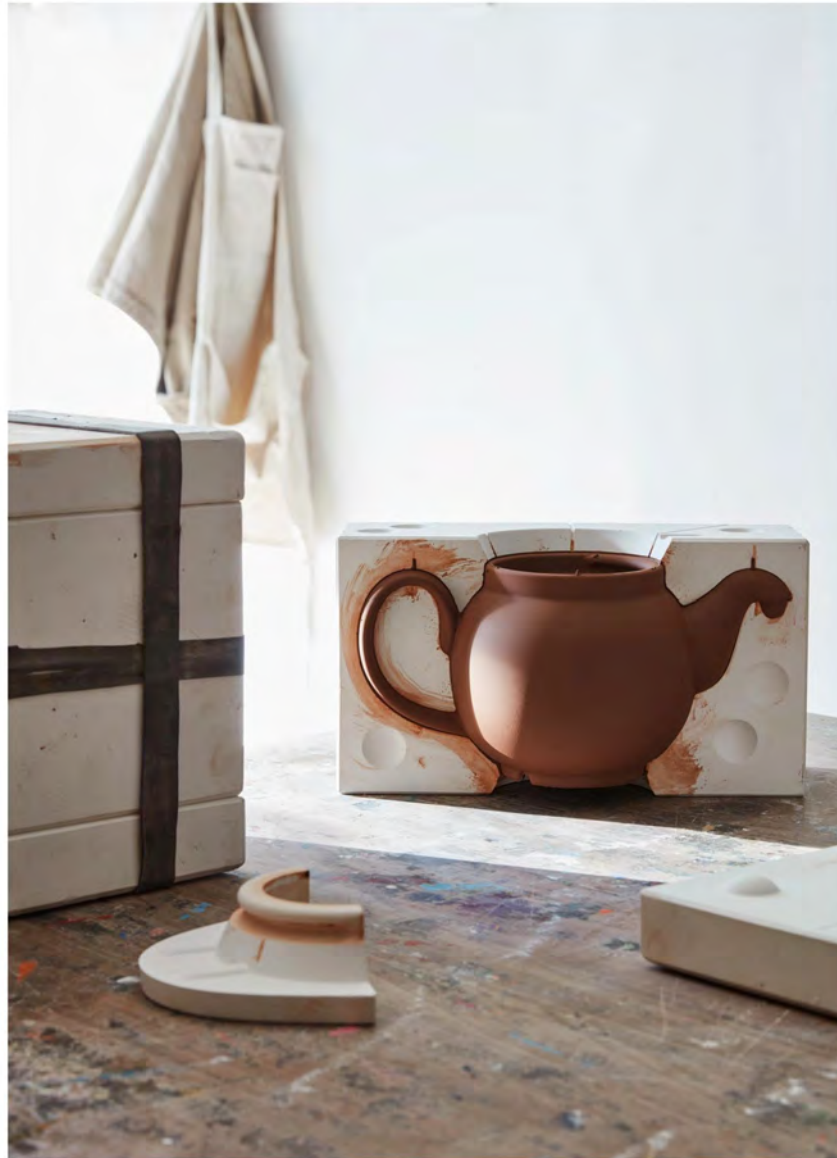
Fig. 129. Air channels allow air to be pushed out of the mould as the slip is poured in; Image Jake Curtis.
