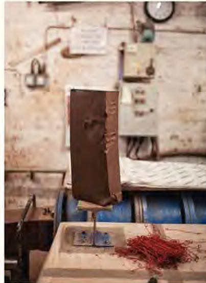
1 An extrusion of Etruria marl clay about to be bagged up by Valentine Clays in Stoke-on-Trent. (Photograph Glen Stoker)
