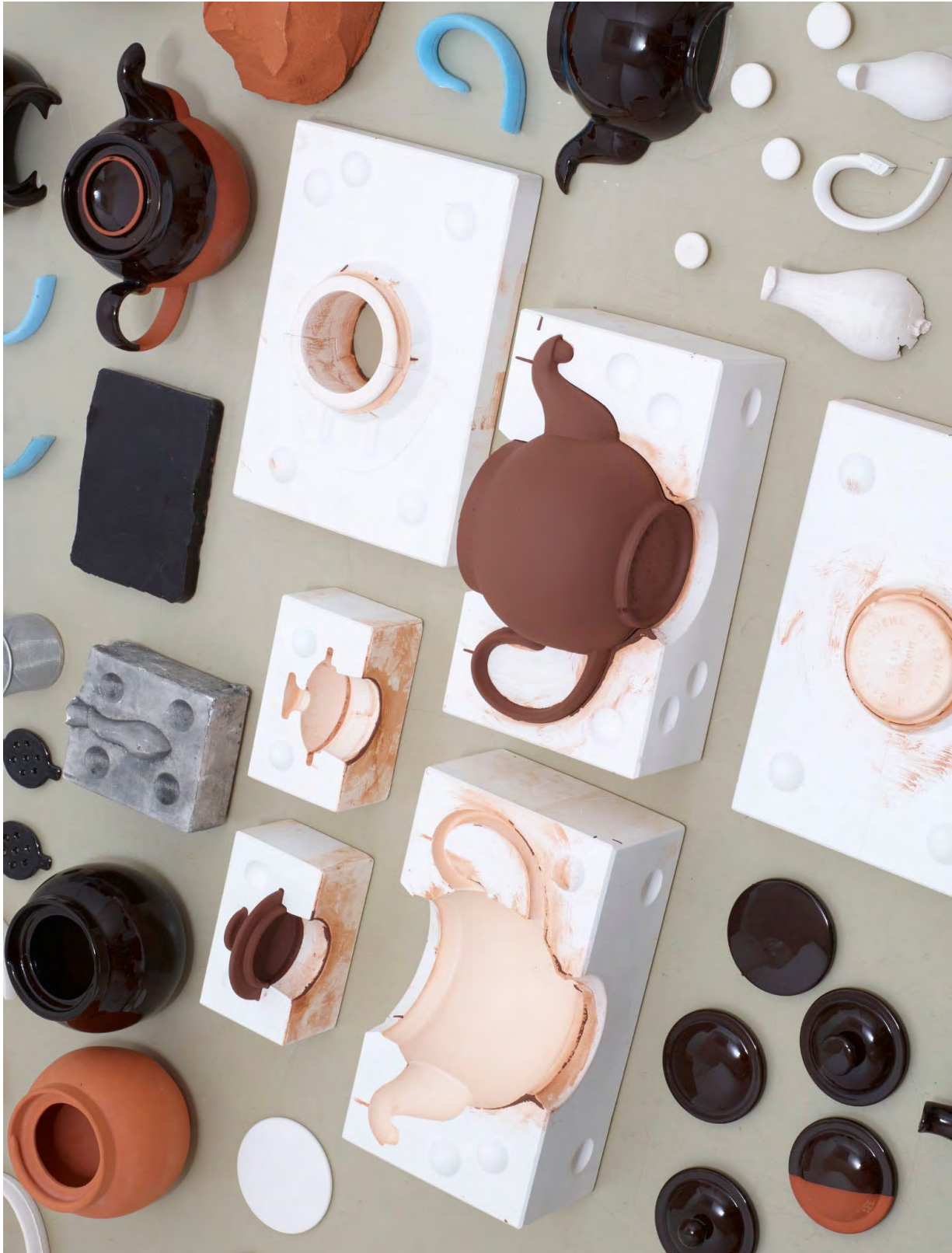
Fig. 141. Models, moulds, material samples and casts laid out as a visual representation of the re-engineering process.
