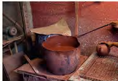
4 At Cauldon Ceramics, a teapot is fettled to remove rough edges before firing. (Photograph Glen Stoker)
