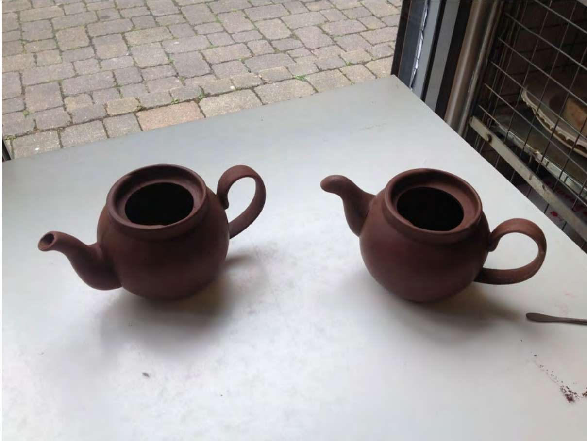
Fig. 124. First casts from the completed handles, globe with locking lid detail and both non-drip and classic spout. Cast in my studio from Etruria Marl clay in moulds made with Ed Bentley.
