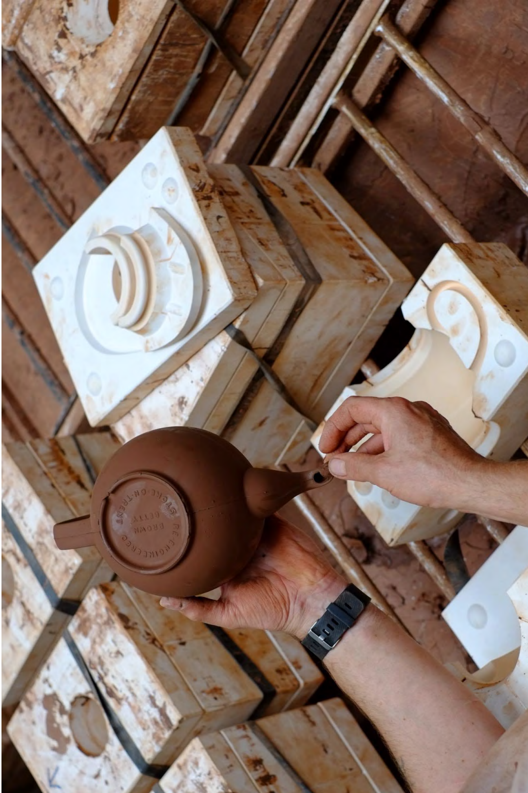
Fig. 132. The embossed makers mark revealed in the cast as it comes out of a new mould at CC; Image Glen Stoker.
