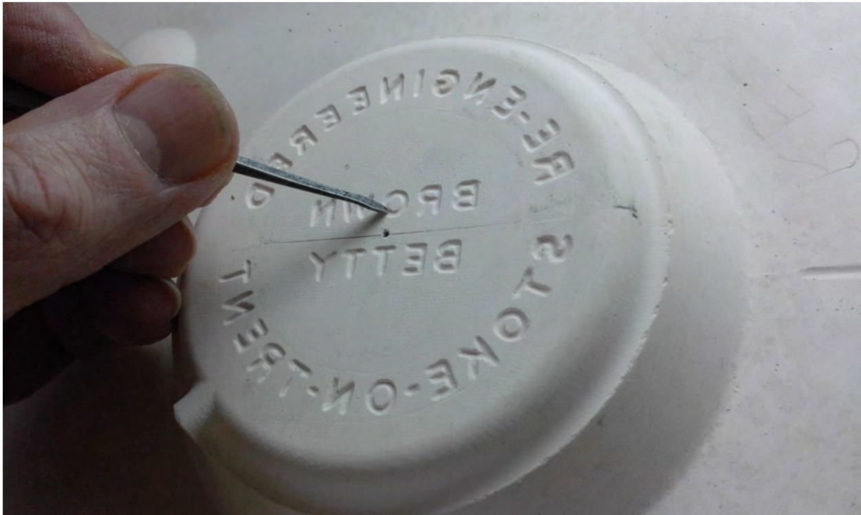
Fig. 131. Ed Bentley scribing a debossed orientation of the makers mark into the master mould in his studio.
