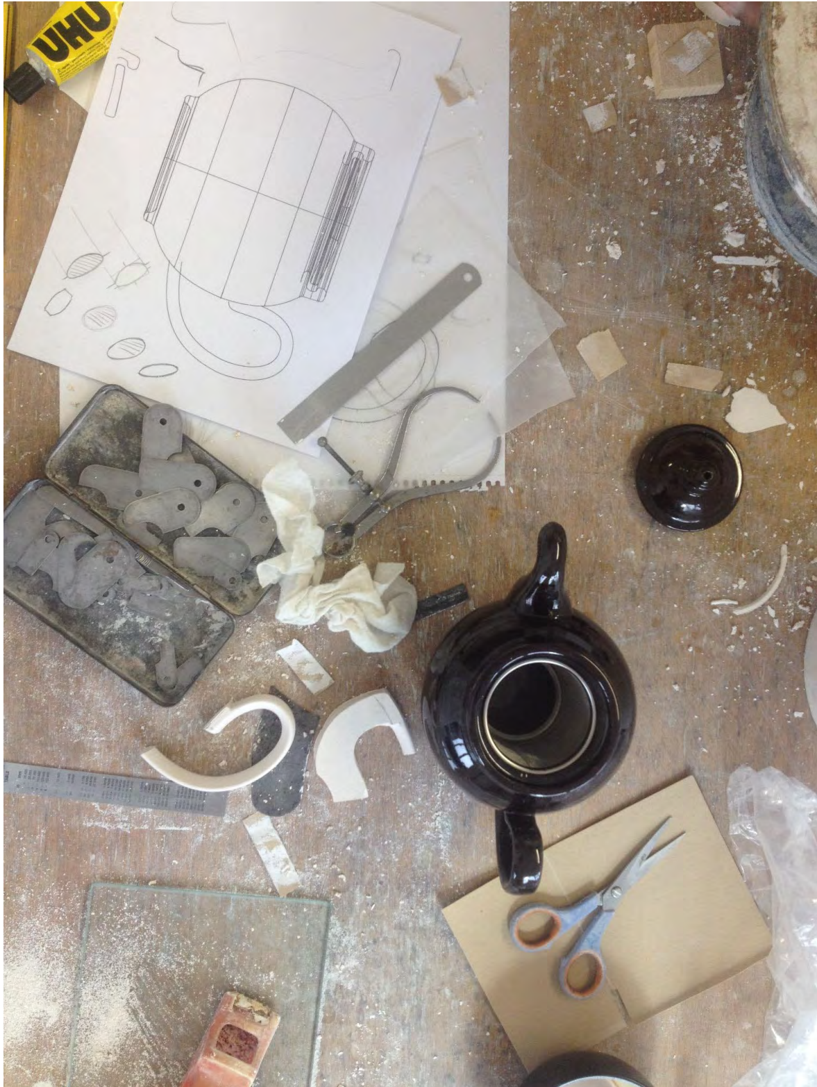
Fig. 130. Working with model maker and historic details and CAD sketch, templates; plaster handle (moving between 2d/3d), to test optimum section thicknesses for handle.
