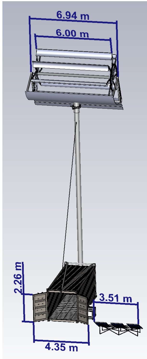
Figure 35: An angled view of the deployed Crossflow turbine CAD file
