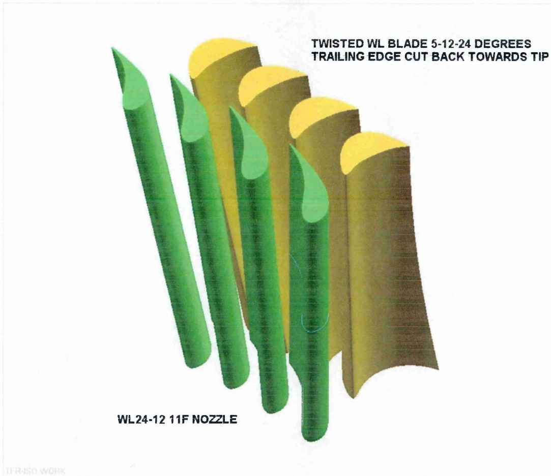
Figure 38. Blade with trailing edge cut back towards the tip.
