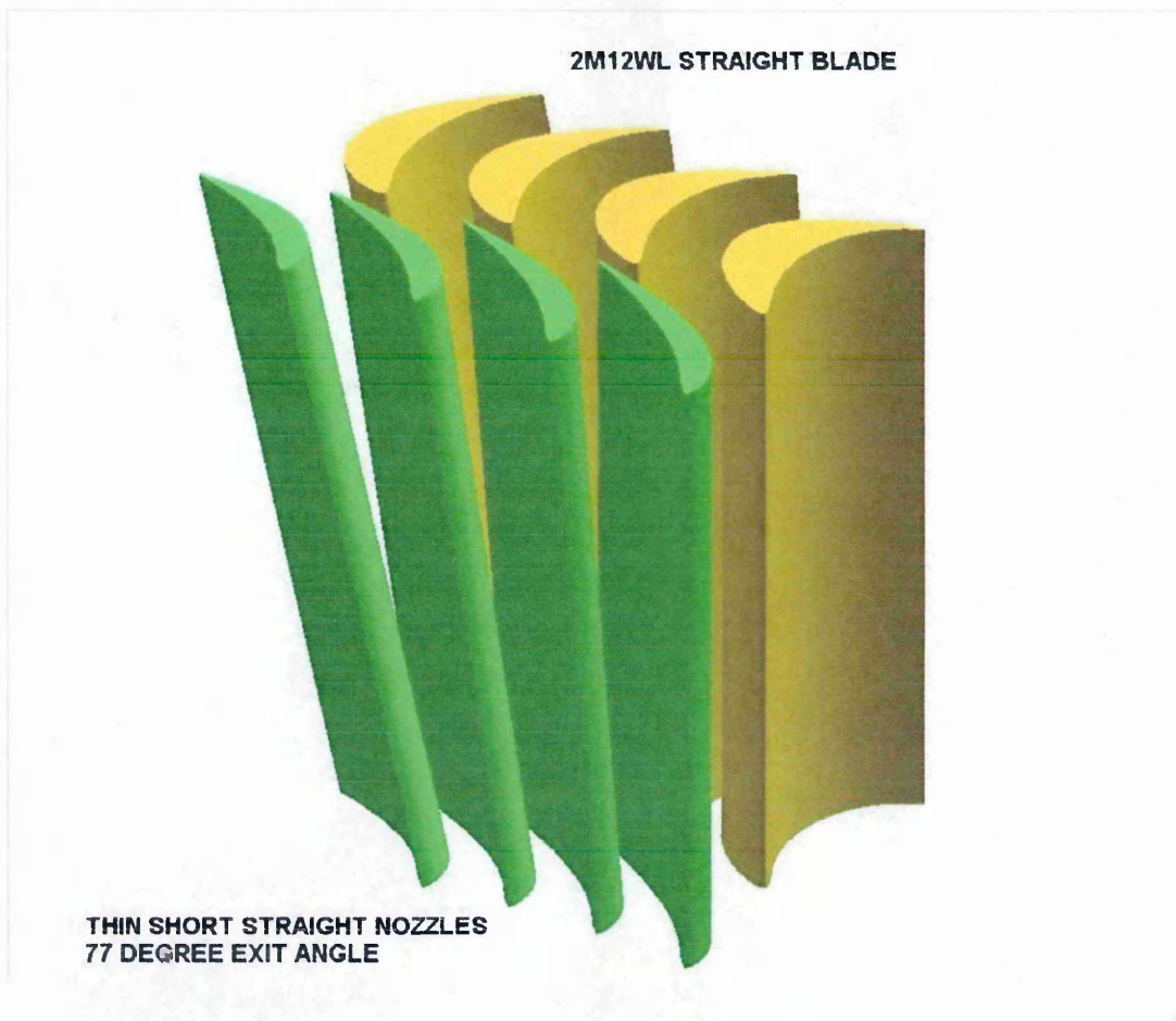
Figure 36. Thin section prismatic nozzles and straight blade.
