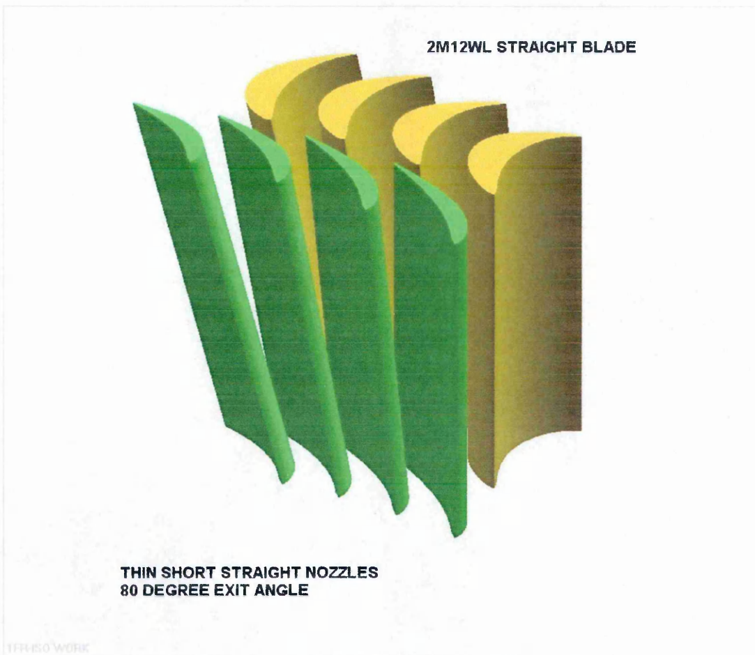
Figure 37. Thin nozzles rotated to 80 degree exit angle.
