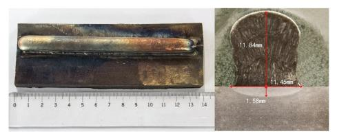
Figure 2-3. Macroscopic morphologies of 308 L stainless steel sample with three layers.
