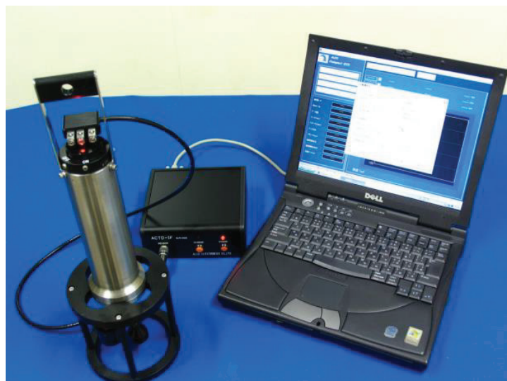
Figure 2.5 Compact CTD (Conductivity, Temperature, Depth) sensor ( Source: JFE advantech Co., Ltd )
