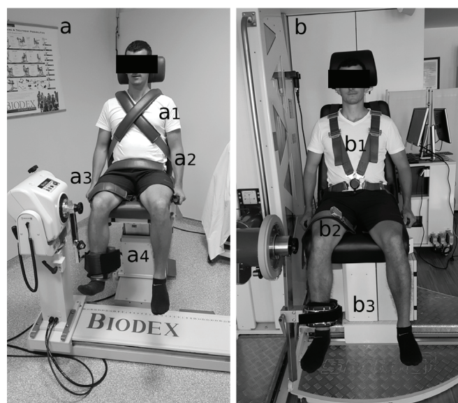
Figure 1. Pictures of both machines and differences between fixation systems: a) Biodex System Pro 4, a1) chest fixation, a2) pelvis fixation, a3) thigh fixation, a4) lever arm fixation and b) SMM iMoment, b1) torso fixation, b2) thigh fixation, b3) lever arm fixation.
