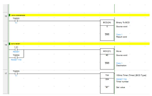
Figure 7. Ladder diagram 2 of detector input
