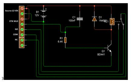
Figure 3. Electronic circuit of WLD
