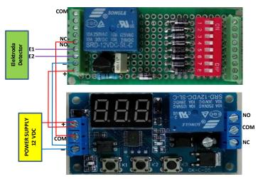
Figure 4. Water level detector
