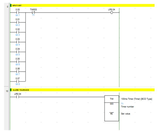
Figure 6. Ladder diagram 1 of detector input
