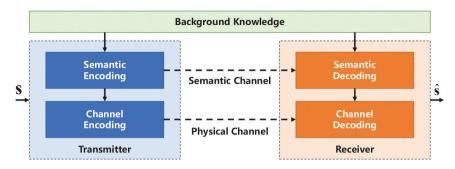
Figure 11: The typical framework of semantic communication system from [103].
