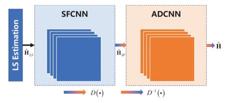
Figure 1: The structure of the dual CNN proposed in [38].
