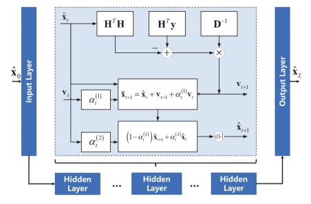
Figure 4: The flowchart representing one layer of the proposed algorithm in [53].
