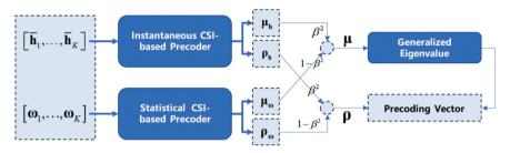
Figure 6: The low-complexity framework for robust precoder design in [80].
