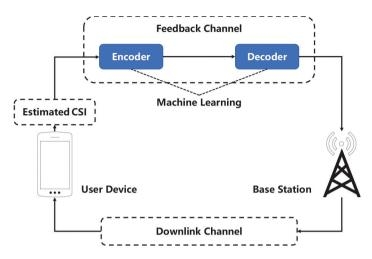
Figure 2: The ML-based CSI feedback.
