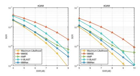
Figure 5: SER performance of different schemes for 4QAM and 8QAM with 16 transmitters, 32 receivers over Gaussian channels in [41].
