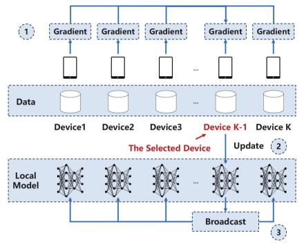
Figure 13: The typical architecture of a fully decentralized FL system.
