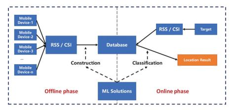
Figure 14: The architecture of fingerprinting-based localization.
