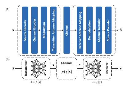
Figure 9: The structures of (a) a traditional wireless communication system and (b) an E2E learning based communication system.
