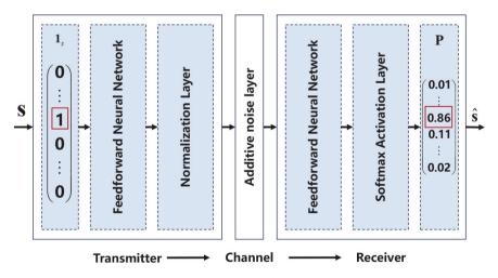
Figure 10: The communications system over an AWGN channel represented as an autoencoder.
