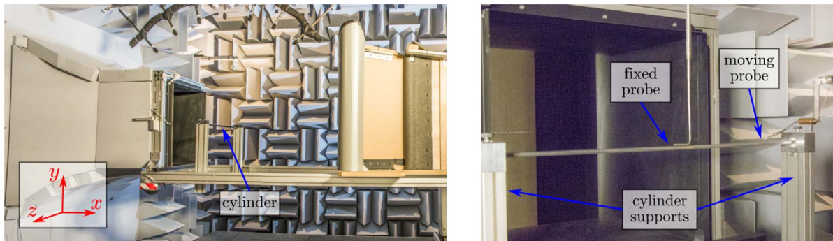
Fig. 1. Wind tunnel facility BETI at Institut PPRIME, at Poitiers, France (left), where the cylinder and hot-wire probes are mounted (right).
