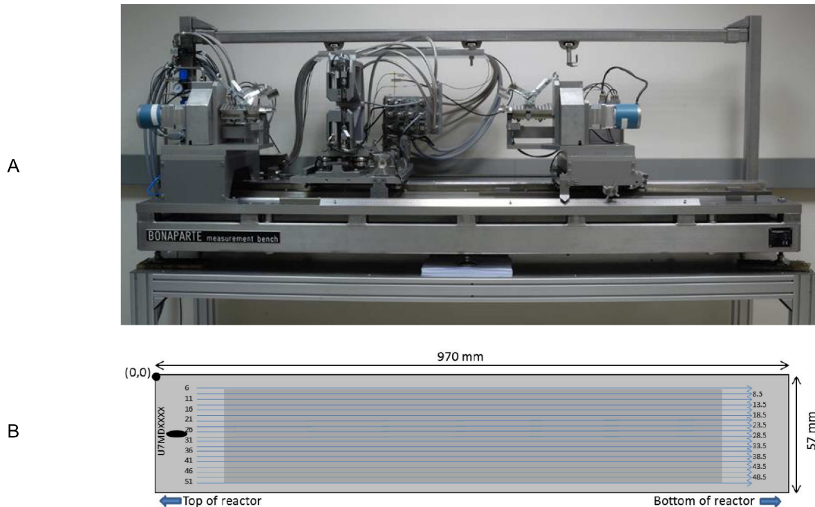
Fig. 5. (A) The BONAPARTE measuring device. (B) Coordinate system adopted for the BONAPARTE measurement results for a typical FUTURE plate.
