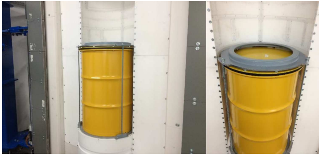
Fig. 5. Universal drum adapter surrounding a drum to be measured.
