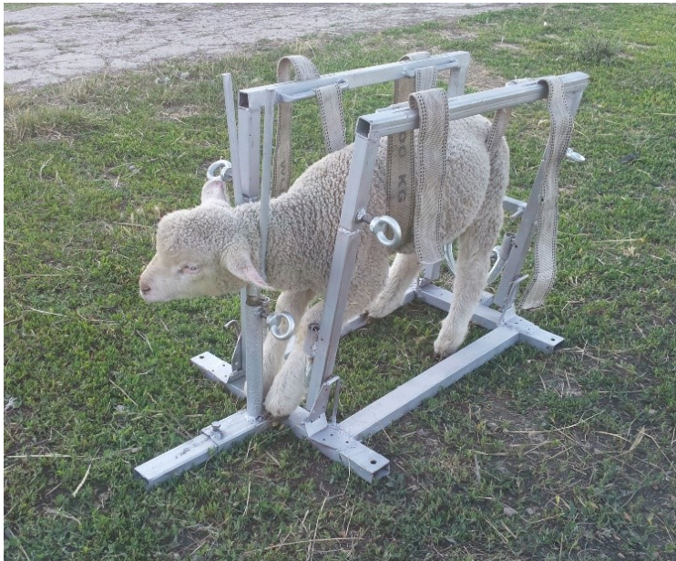
Fig. 6. A device for fixing sheep and lambs with the possibility of using low-intensity laser radiation.
