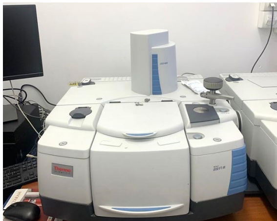
Fig. 1. Nicolet iS 50 FT-IR Spectrometer, with Built-in mid- and far-IR capable diamond ATR
