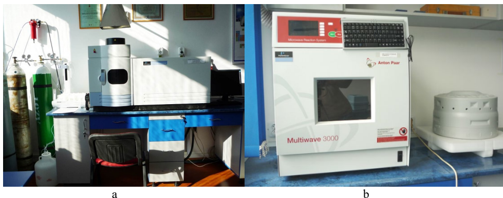
Fig. 2. a. Inductively coupled plasma optical emission spectrometer ICP-OES Perkin Elmer: b. Microwave oven for solid sample digestion
