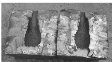
Fig. 5. Lead cylinder sectioned after Trauzl test with explosion results.
