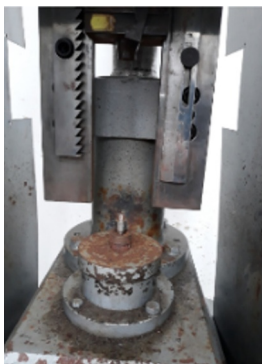
Fig. 3. Placement of the impact device filled with the explosive substance sample in the impact test equipment.
