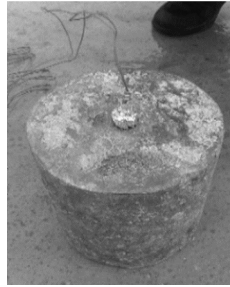
Fig. 1. Cylindrical lead block, TNT explosive assembled in cartridge and primed with detonating electric detonator.
