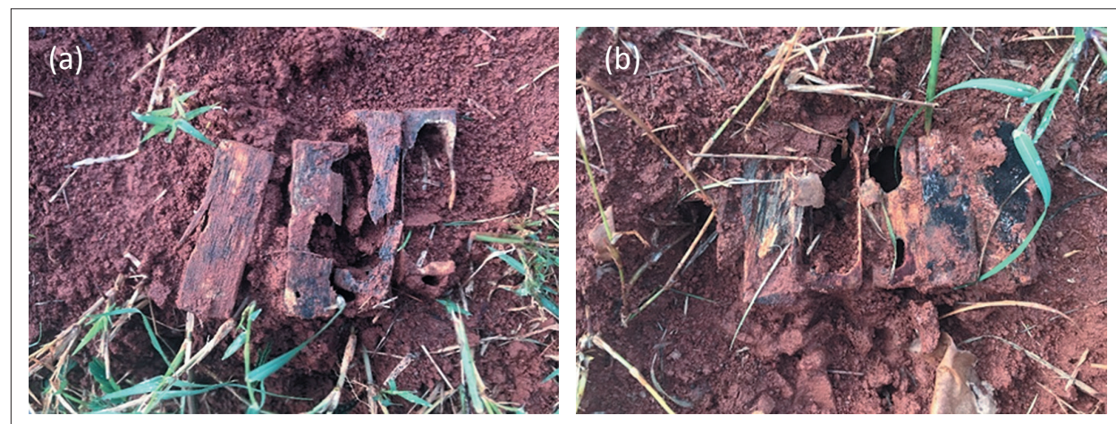
Figure 5. Ayous ( Triplochiton scleroxylon ) wood impregnated with NO 10% (a) and NO 30% (b) after 16 weeks in a termitarium.
